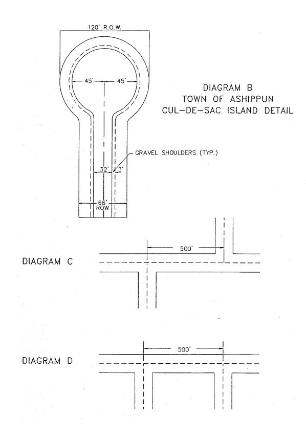
Arterial Streets: Five Hundred (500) Feet Collector Streets: Three Hundred (300) Feet A tangent at least one hundred (100) feet in length shall be provided between reverse curves on arterial and collector streets.
